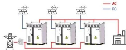
Parallel (Parallel operation up to 6 unit (only with battery connected))
