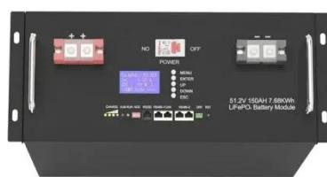
51.2V 150AH, 7.68KWH
