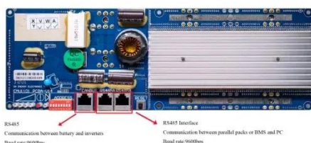
RS485 Communication between battery and inverter Band rate 9600bps
